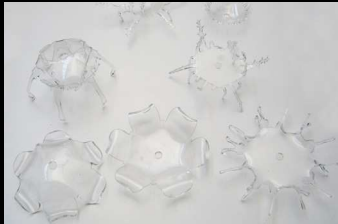
Lasercut and thermobent acrylic lenses
