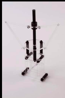
Kinetic design: umbrella with scotch yoke
