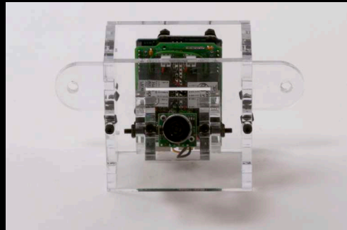
Circuit with ultrasonic sensor and microcontroller in wall mount
